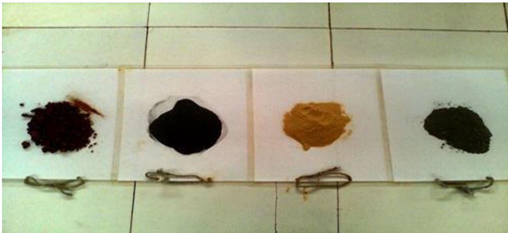
Fig. 1: Laterite, rice husk ash, glass powder, and cement samples
