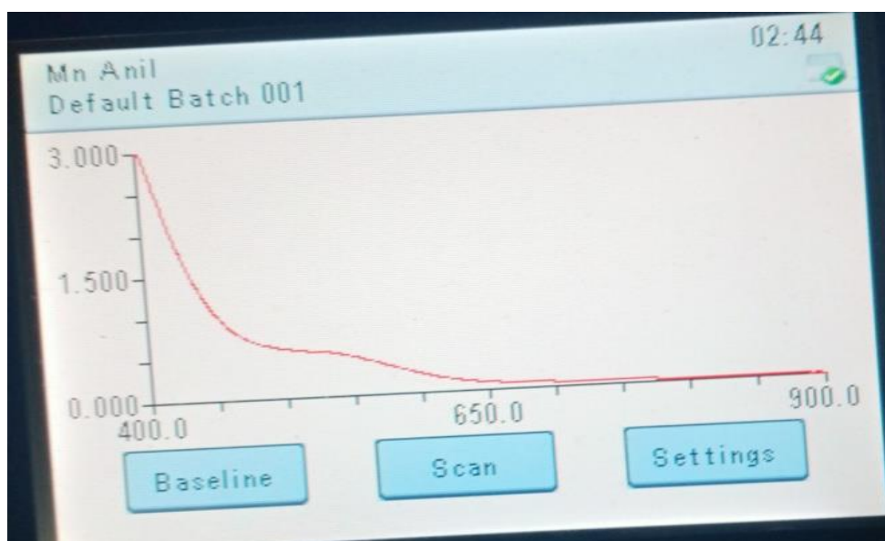
UV visible spectrum of \text{Mn}(\text{C}_7\text{H}_7\text{NO}_3)_2(\text{C}_6\text{H}_7\text{N})_2
