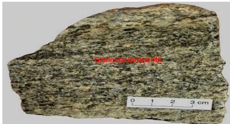
Fig .9: Granites sample Methods Laboratory analysis Petrographic analysis of the rock samples using Dave's method
