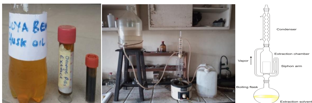
Plate 3: Soya bean husk oil, orange peel oil and Soxhlet and schematic of Soxhlet extractor
