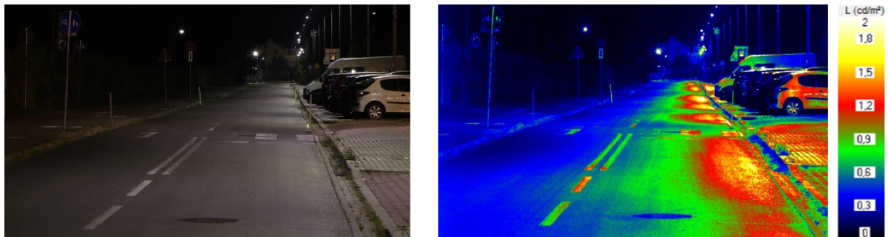
Fig.1. Left picture shows the street picture, and the right picture shows the luminance distribution
