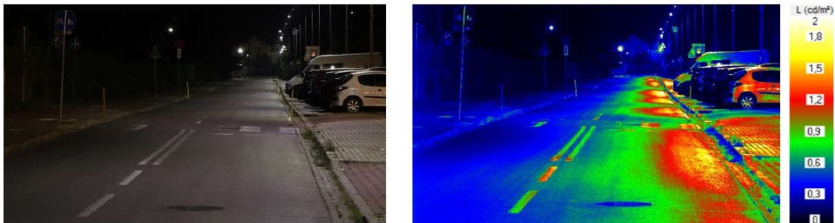
Fig.2. Left picture shows the street picture, and the right picture shows the luminance distribution
