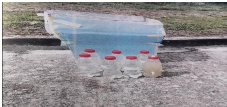
Figure 4. Diagram of a constructed solar disinfectant and the samples of water.
