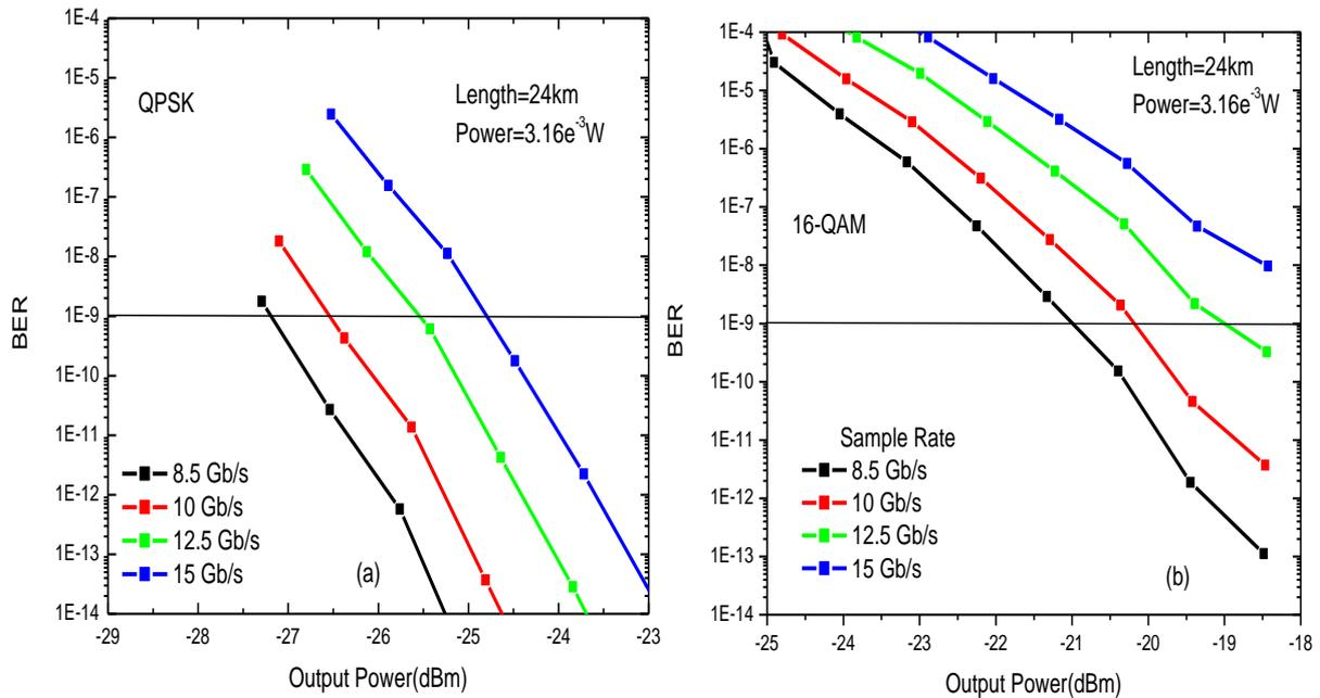
**Figure 4: Characterization of optical signal transmission using; (a) QPSK (b) 16-QAM modulation formats**
