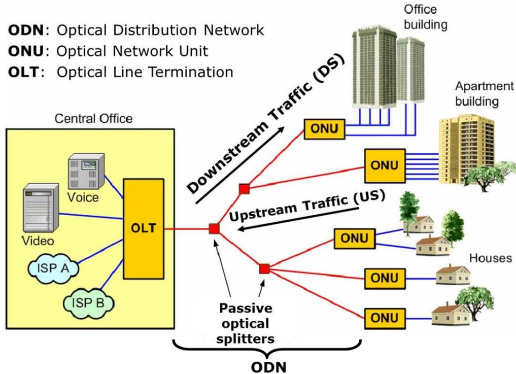
**Figure 1: Passive optical network architecture [9]**
