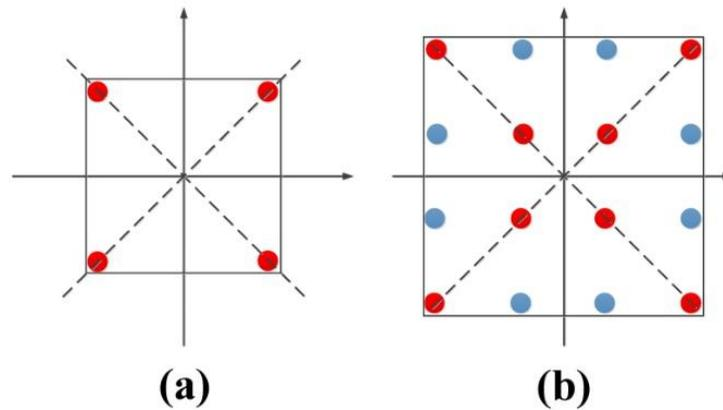
**Figure 2: Constellation of (a) QPSK (b) 16-QAM**
