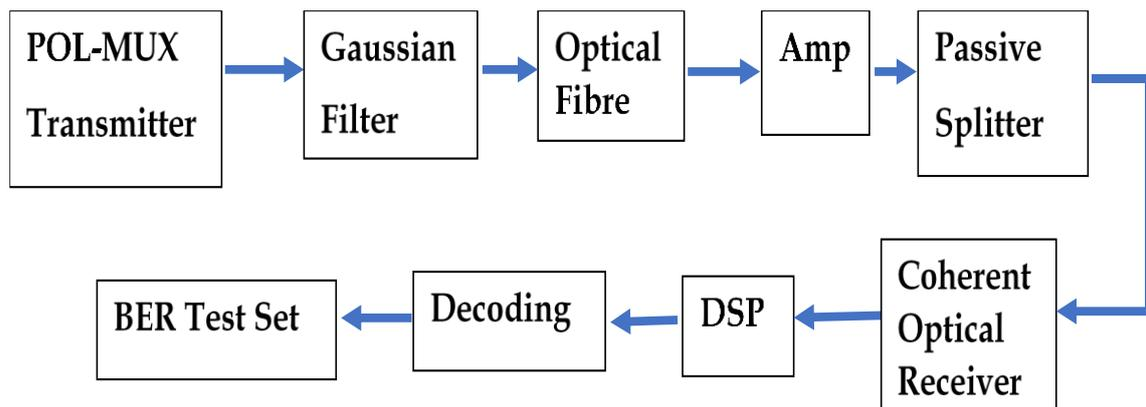
Figure 3: The block diagram of DP-QPSK and DP-16QAM transmission system.
