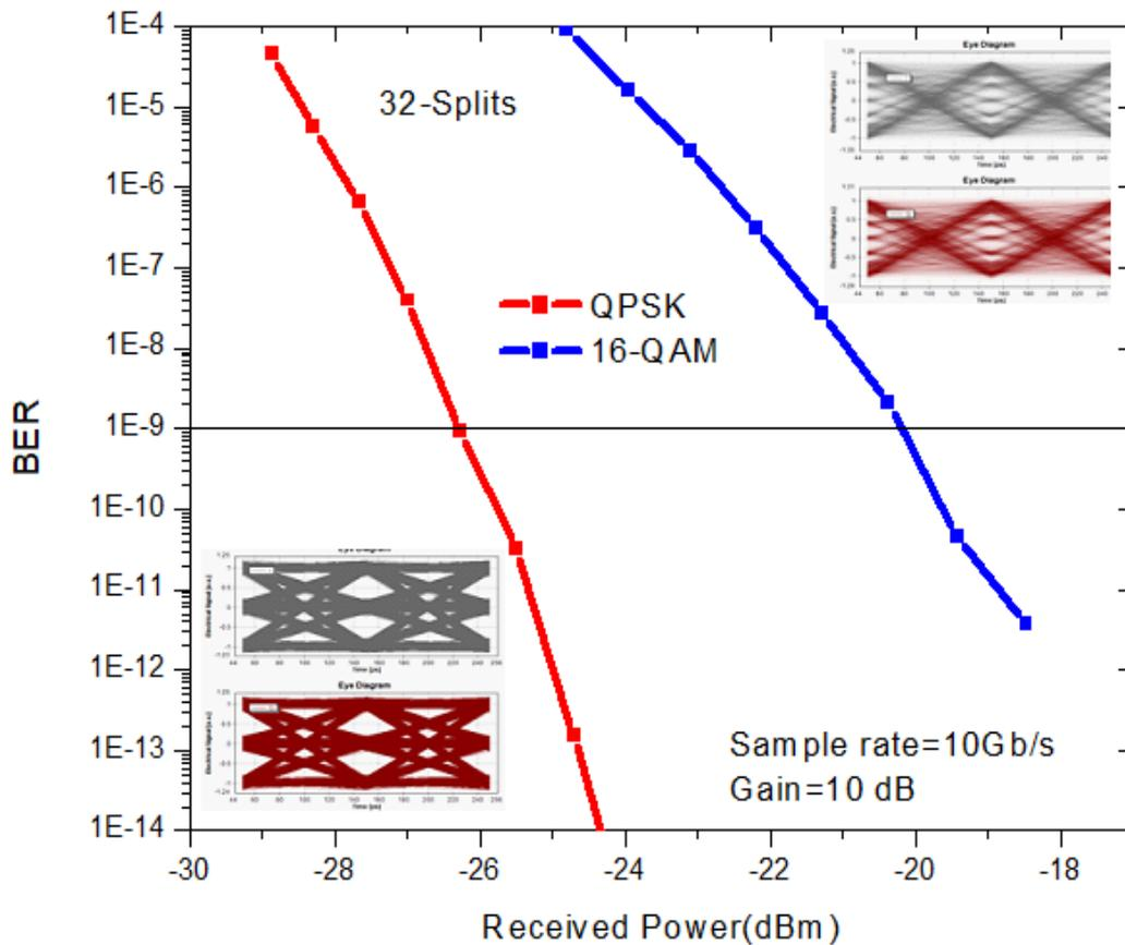
Figure 5: BER curves for QPSK and 16-QAM for 32-Splits. Inset: Respective eye diagrams.
