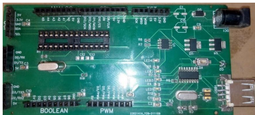
Figure 2: Printed Circuit Board for the novel Prototyping Development Board (Bottom circuit connections are colored GREEN)
